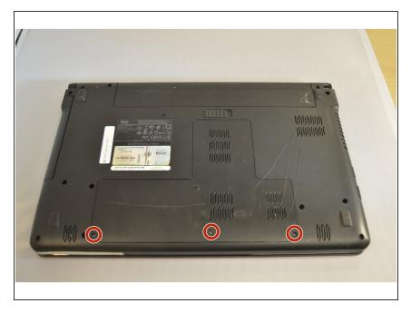
With a J0 screwdriver bit, loosen all screws from the backing above the battery latch and remove the covering.
