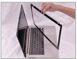
Remove display screen frame completely before adhesive cools and hardens.
