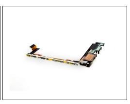
Loosen side button contactors (Attention: the fingerprint sensor is here, be careful to loosen it),
