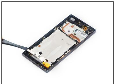
Remove the metal bracket covering on the LCD screen flex.
