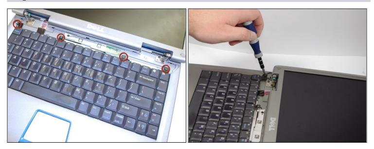
• Using a Phillips screwdriver remove the four M2 x 3-mm screws holding in the keyboard.
