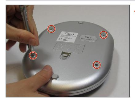
Using a 2.0 Flathead screwdriver, remove the four
