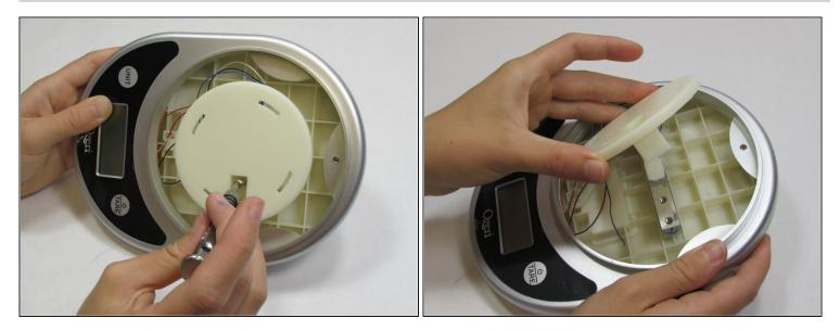
• Using a 2.0 Flathead screwdriver, remove the two 18.76 mm Phillips head screws in the plate stand.
