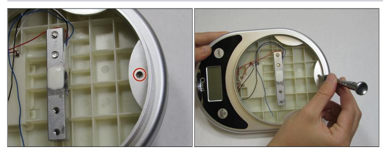
• Using a 2.0 Flathead screwdriver, remove the 9.44 mm Phillips head screw on the edge opposite to the LCD screen.
