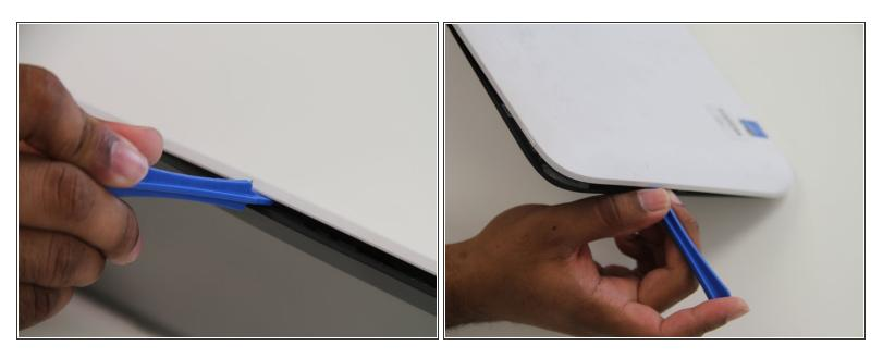
• Use a plastic opening tool to pry the tabs on the top, left and right sides of the tablet.
