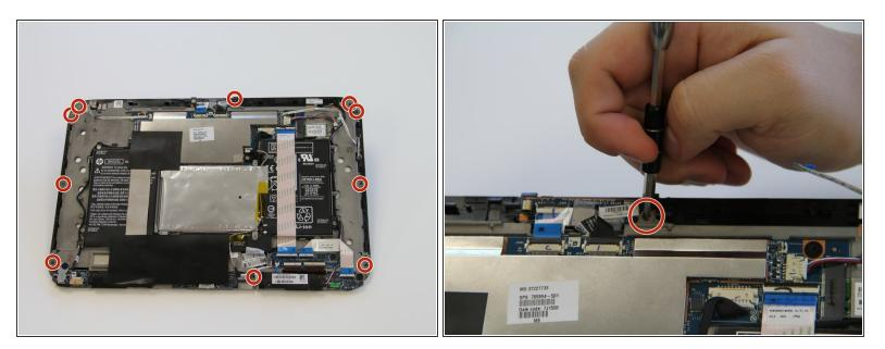
Use a J0 screwdriver to remove the ten 4mm Phillips screws.
