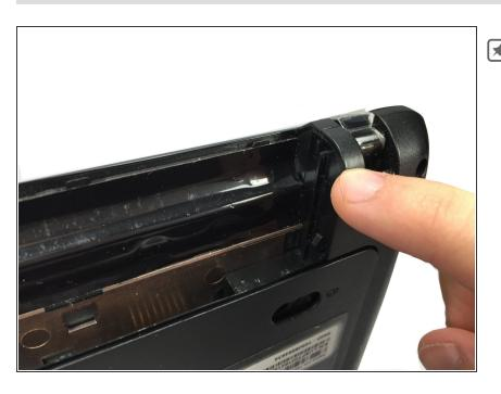
Check the thin grooves on the side of the battery entry and line the replacement battery up to the grooves.
