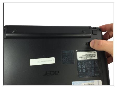
Slide the button below the battery to the right while simultaneously pulling the battery out.
