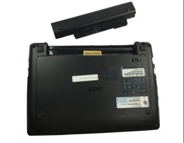
If necessary, remove the old battery and replace it with a new one.
