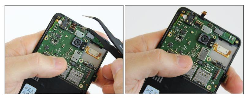
• Using one prong of the tweezers, pry the ribbon clip away from the motherboard.
