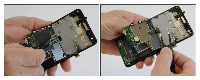
Using one prong of the tweezers, lift and pry back the metal clip positioned over the front proximity sensor ribbon connector.
