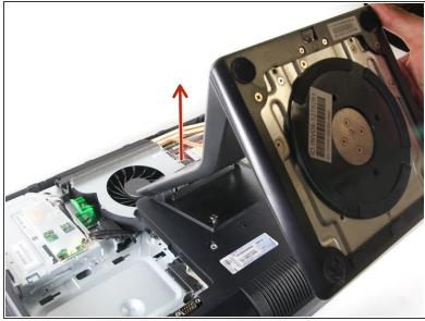
Loosen the two 1/2" screws, with the T15 Torx Screwdriver, on each side of the stand. Remove stand.
