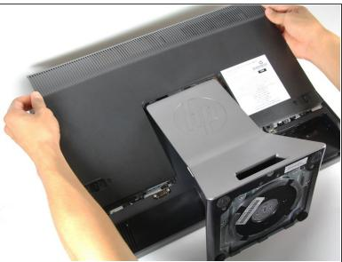
Push the unlock tabs on the back of the monitor in and towards each other while sliding the back cover up.
