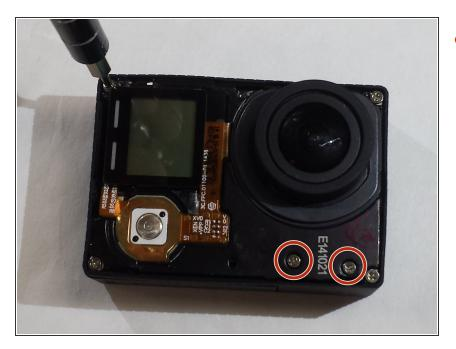
Remove these two screws and remove the riser that is being held in by the screws.
