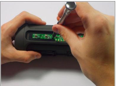
Unscrew the 2 screws that hold the circuit board in place.
