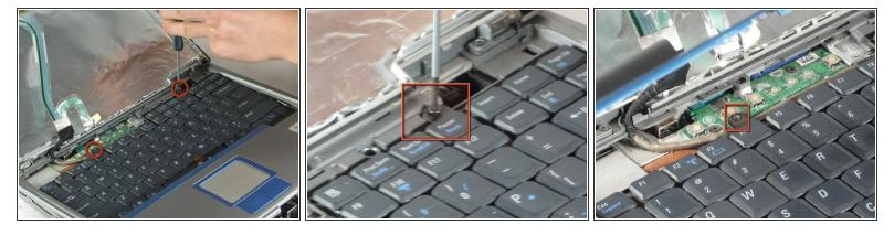
Use a the Phillips screwdriver to remove the two screws.
