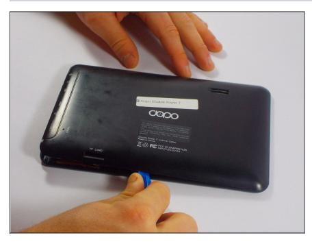
Run the plastic opening tool along the seam looking for the clips and lift up on the rear panel.
