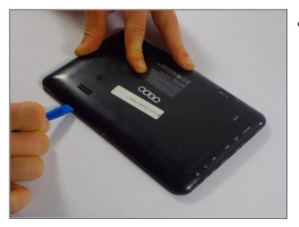
• Carefully, wedge the plastic opening tool in-between the seam that separates both halves of the tablet.
