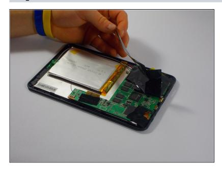
• Remove any static tape covering the motherboard.
