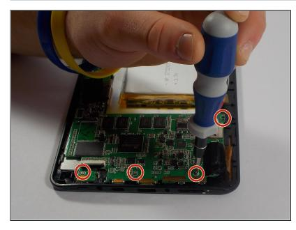
Using a Phillips Head Screwdriver size 0, remove the four screws attaching the motherboard.
