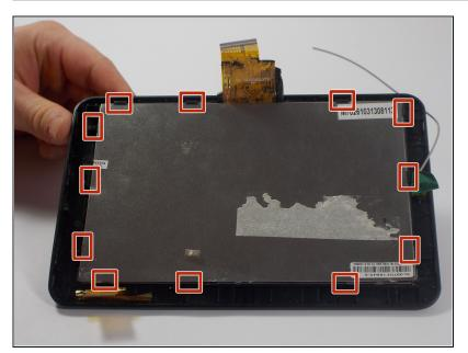
The back of the digitizer is attached along the edge by 12 plastic clips.
