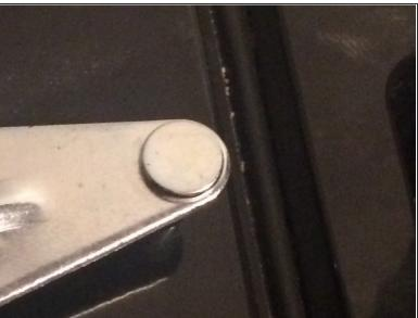
Remove the damaged hinge. Make sure that you don't lose the bolt that goes into the door.
