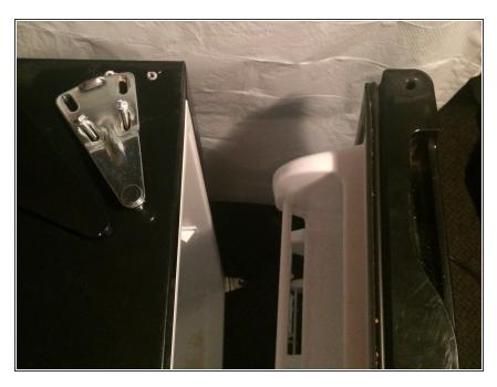
Remove the door by slowly lifting straight up, put the door off to the side.
