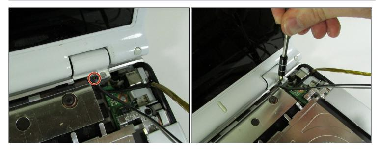
• Use a Phillips #00 screwdriver to remove the black screw located in the top right corner near the display.
