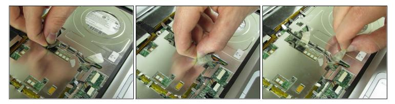
• Pull up on tape holding down wires.
