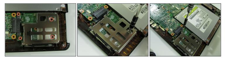
• Remove the four screws from the ExpressCard component using the Phillips #00 screwdriver.
