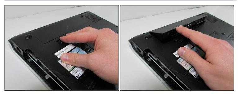
• Slide the tab all the way over to the left until battery pops out. Lift out and remove battery.
