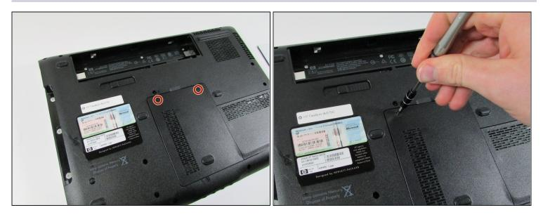
• Remove the RAM port cover by unscrewing the two screws.
