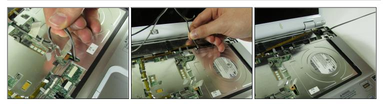
• Pull up on the WiFi wires and out from under the metal tabs.
