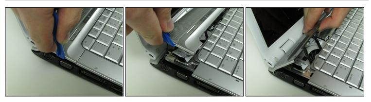
Use an iFixit opening tool to pry open the plastic bar above the keyboard.
