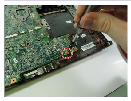
Using the Phillips #00 screwdriver, remove the one screw near where the ExpressCard component was.
