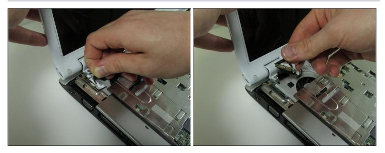
• Pull upward on the screen connector tab.
