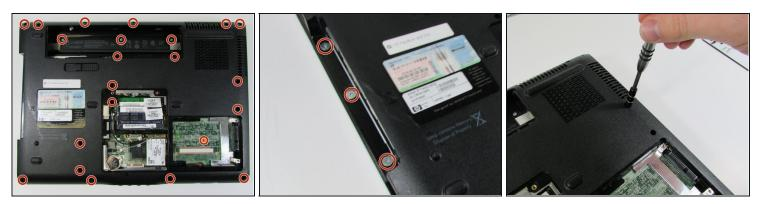
• Use a Phillips #00 screwdriver to remove the 25 screws securing the bottom of the computer.
