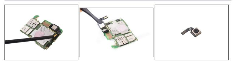
• Release rear camera contactor, then remove it.
