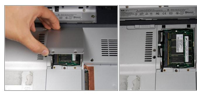
Lift up on the screw side of the RAM access cover to remove it.
