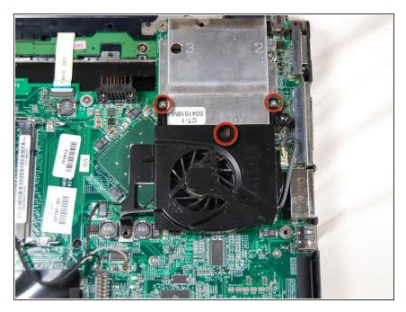
Remove the highlighted screws with the #00 Phillips screwdriver.
