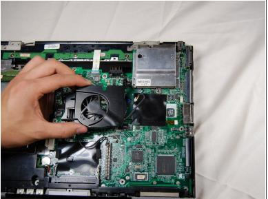
With the wire removed, the fan should lift up easily from the board.
