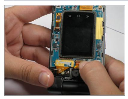
• Close the tab down onto the new camera ribbon.
