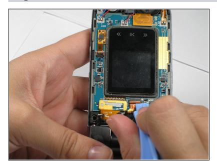
• Use a plastic opening tool to lift the tab that holds the camera ribbon in place.
