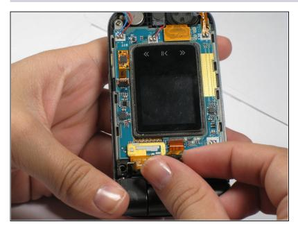
• Slide ribbon of new camera under the same tab.
