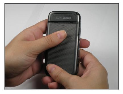
• Push down on the back cover of the phone, then remove the back cover.
