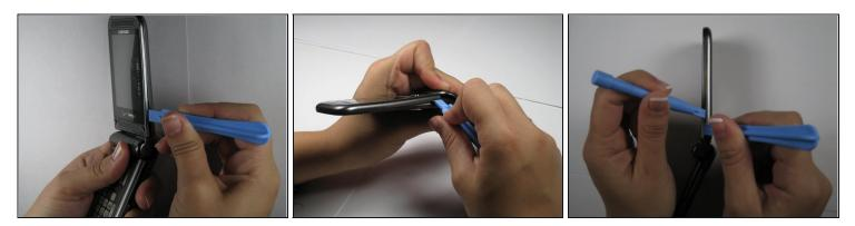
• Remove front outside casing with plastic opening tools.
