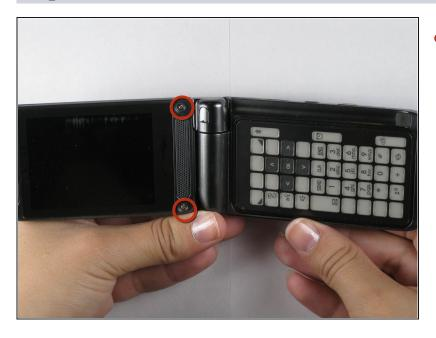
• Remove the (2) 4.1 mm screws on screen.
