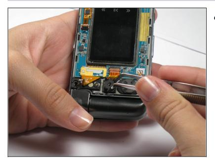
• Use tweezers to remove the camera from its holding slot.
