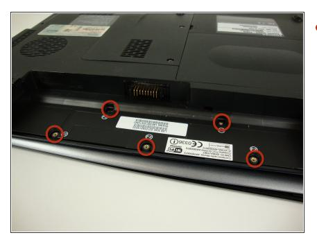
Remove the five "F2" screws with a Phillips #0 screwdriver.
