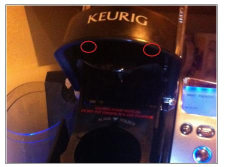
Point the tip of your Philips-head screw driver up and remove the two screws on the underside of the head. (circled). Be careful you don't drop and lose them!
