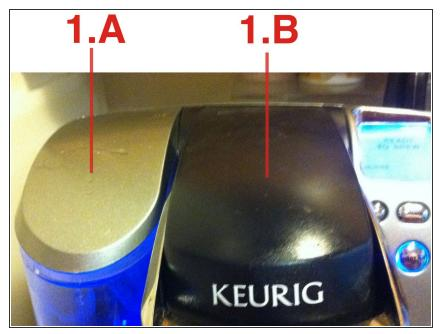
Identifying the parts: 1.A is the water reservoir cover. 1.B is the "Head". The needle that punctures the K-Cup is in here.
