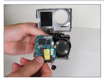
• Fully remove the motherboard from the camera body.
