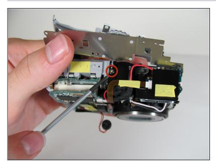
• Remove the 2.8 mm screw from the top of the camera.
