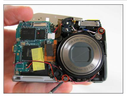
Remove the two screws on the opposite sides of the flash.
