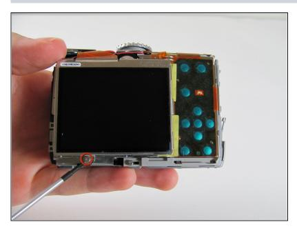
Remove the 3.1 mm screw below the LCD.
