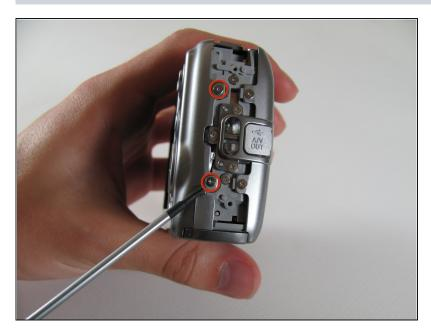
Remove the two 4.8 mm screws attaching the back panel to the body on the left side.
