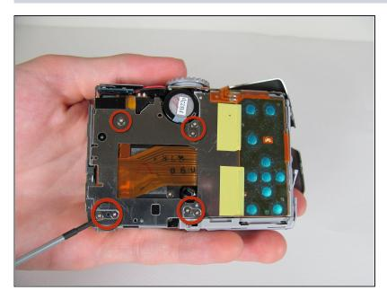
Remove the seven 2.8 mm screws from the back of the camera.
