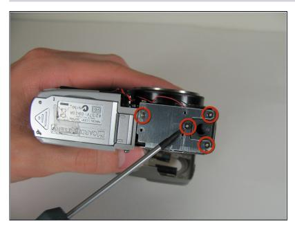
Remove the four screws on the bottom of the camera.
