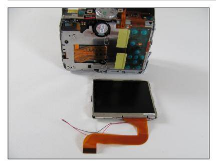
Remove the LCD from the camera body.
