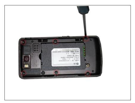
Six Phillips screws holding down the battery housing (Circled in the picture). Unscrew the six screws and put them aside.
