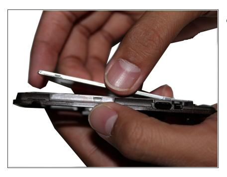
Remove the broken LCD Screen from the housing.
