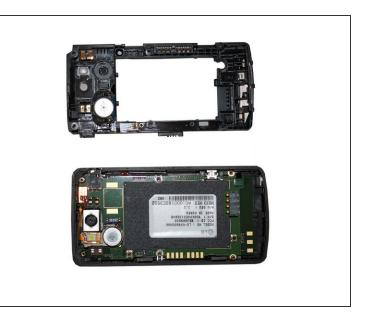
Insert a safe prying tool between the slot between the front screen housing and the battery housing to remove the battery housing.
