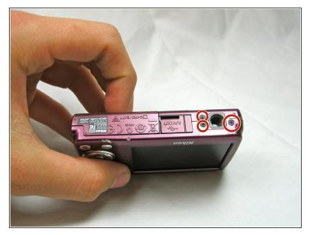
• Remove the three 4.1 mm screws on the bottom of the camera.
