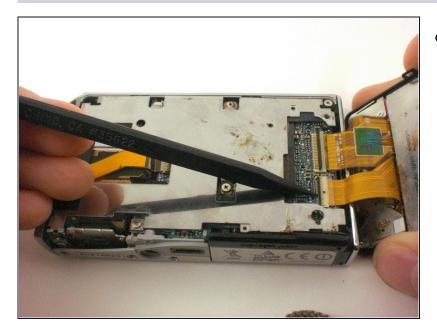
• Lift the back cover, being careful not to rip the orange cables between the camera and the back cover.
