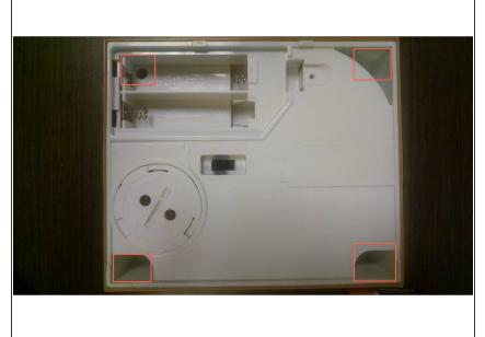
Remove the four screws holding the cover in place. You'll need a traditional Phillips screwdriver, not a screwdriver set, to reach fully into the wells.
