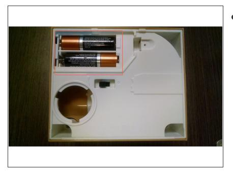
Remove the battery cover and batteries.
