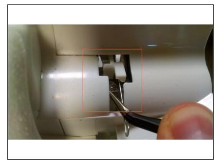
Remove the coin using a set of tweezers.
