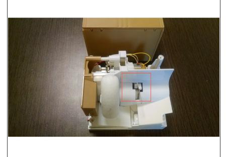
Locate the jam. You might need to temporarily put in the batteries to activate the arm, so you can find the jam.
