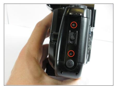
Remove two 6.4mm screws on the latch mechanism on the right side of the camera.
