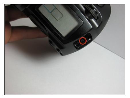
Remove the 4.3mm screw below the camera strap ring.
