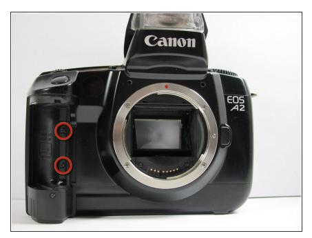
Remove the 5.6mm screws behind the battery cover.
