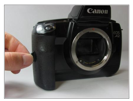
Locate the battery door/camera grip on the left side of the camera and lift the rotating removal tab.
