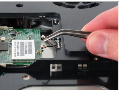
Use tweezers to detach the grey and black cables connected to the green WiFi card.
