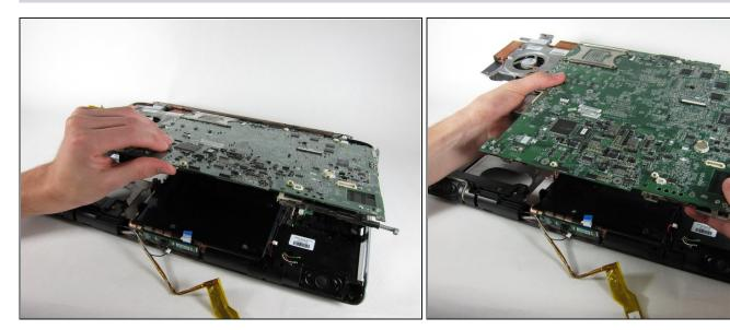
• Lift the motherboard up until it releases from the bottom casing and remove it from the laptop.
