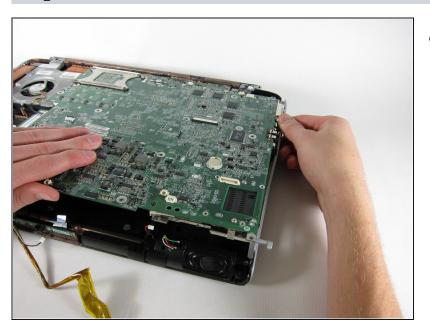
Pull the right casing to the side to release the ports on the motherboard from it.
