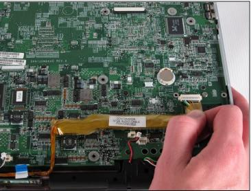
• Remove the audio cable - the one with the yellow covering located at the bottom-right corner of the motherboard - by pulling the yellow covering towards you.
