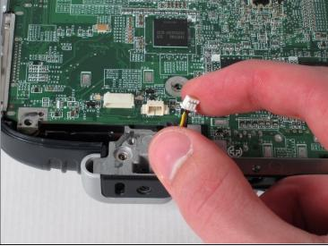
• Remove the fan cable by pulling the white connector away from you.
