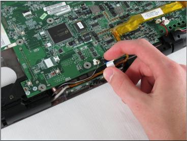
• Remove the LED board cable by pulling the white tab towards you.
