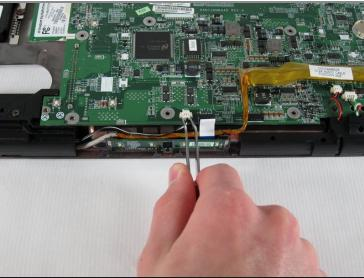
• Using tweezers, remove the left speaker cable by pulling the white connector towards you.
