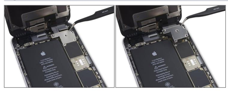
• Remove the display cable bracket.
