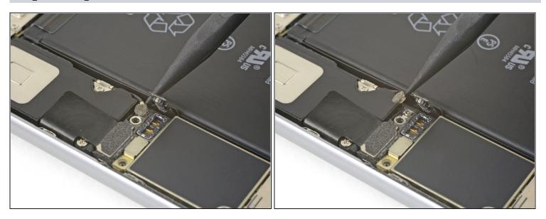
• Use the point of a spudger to pry up and disconnect the antenna cable from the bottom of the logic board.
