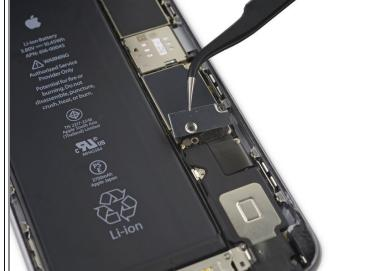
• Remove the battery connector bracket.
