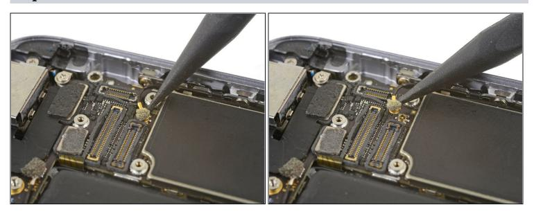
• Use the point of a spudger to pry up and disconnect the antenna cable from the top of the logic board.
