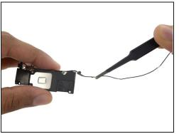
• Use a pair of tweezers to begin peeling the antenna cables off of the speaker.
