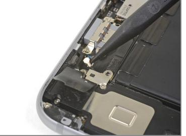
• Use the point of a spudger to pry up and disconnect the antenna cable from the Lightning connector assembly.
