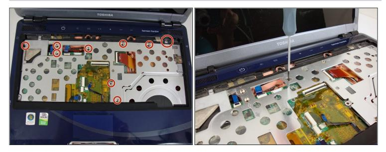
• Remove the circled screws with Phillips #0 screwdriver.
