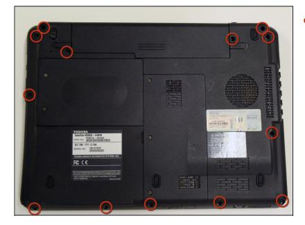
Remove these screws from the underside of the laptop with Phillips #0 screwdriver.
