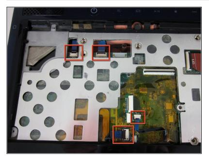
Detach the four blue ribbon cables carefully with <u>tweezers</u>. Some of the ribbons may require a flap to be raised because it secures the ribbon in.
