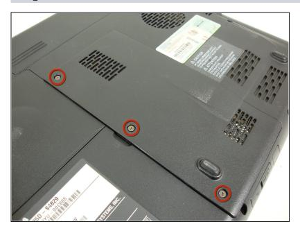
Remove the back panel by removing the three labeled screws with a Phillips #0 screwdriver.
