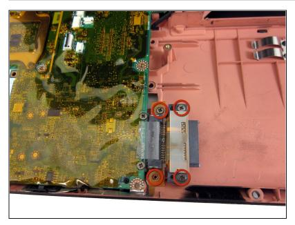
• Remove these screws with a Phillips #0 screwdriver.
