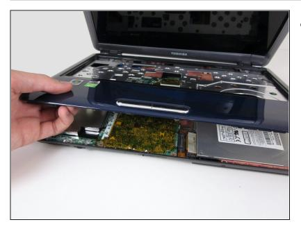
• Remove the top plastic cover by lifting upward from the bottom left-hand corner as shown. The cover will come off easily.
