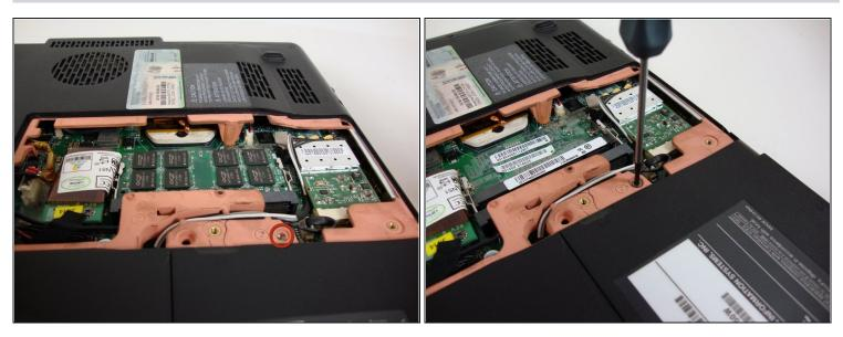
• Locate and remove the circled screw with a Phillips #0 screwdriver.
