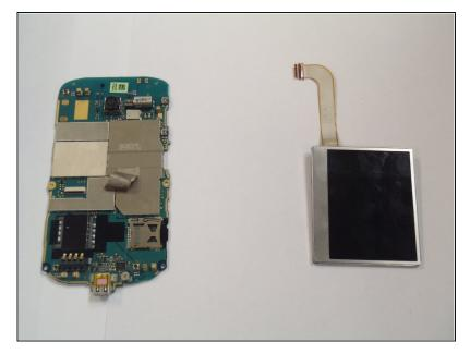
• Lift the Motherboard away from the LCD display.
