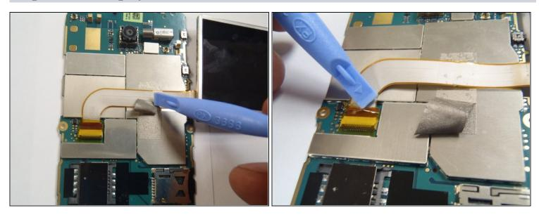
• Remove the gray tape securing the ribbon cable.
