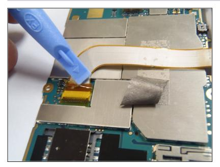
Remove the yellow tape securing the connector lock.
