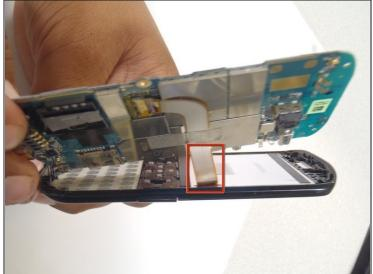
Pry the motherboard away from the front of the plastic case using a plastic opening tool.
