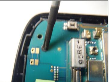
Remove the single Phillips #0 screw that is securing the motherboard to the front case of the phone.
