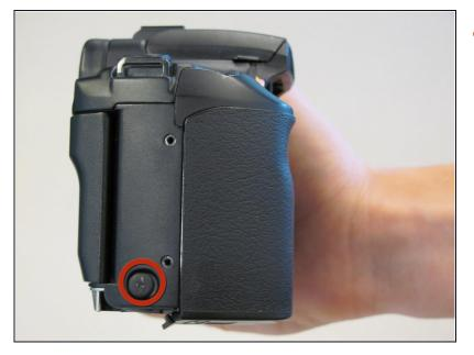
Remove the plastic remote control socket cap by pulling it straight out.
