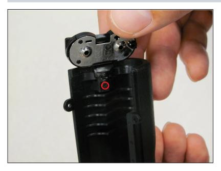
• Remove one black screw from battery door on underside of grip.
