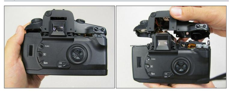
• Slowly separate the top panel from the camera by pushing it upward.
