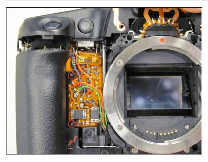
• Remove the two 5.5 mm screws from front of camera.
