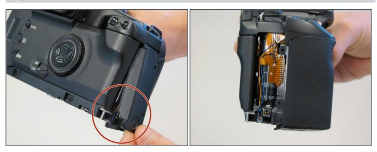
• Slide the panel toward the bottom of the camera to remove.
