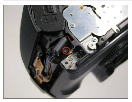
• Remove the single 4.8 silver screw from the control socket.
