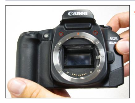
• Remove the two 4.8 mm black screws above the lens on the front of the camera.
