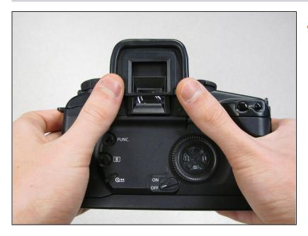
• Slide the outer eyepiece upward to remove it.
