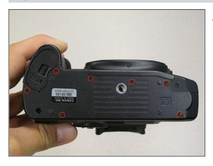
• Remove seven 4.25 mm black screws on the bottom panel.
