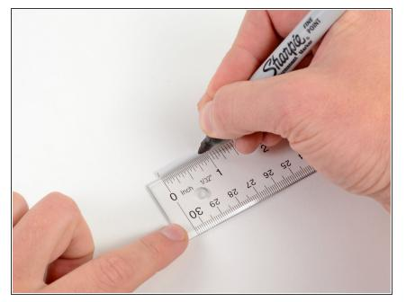
Use a pen to make a mark about .75" (2 cm) from the cut end on the side of the cable attached to the power adapter.
