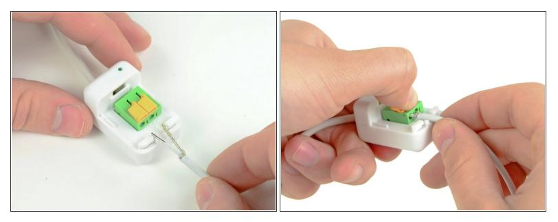
• As in step 13, use your thumb to push back the orange spring clamps on both terminals and insert the center wire into the positive (+) terminal on the left and the outer wire into the negative (-) terminal on the right.
