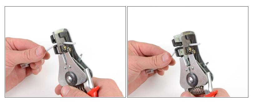
Again, use the largest (innermost) stripping hole to remove the outer cord tubing at the mark you
