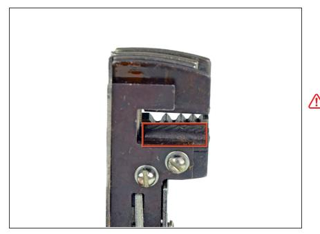
Before using the included wire strippers, we recommend cleaning the upper and lower flat areas where the tool grips the cable with degreaser. The manufacturing process leaves a small amount of grease on these areas that may stain the white cable you are about to strip.
