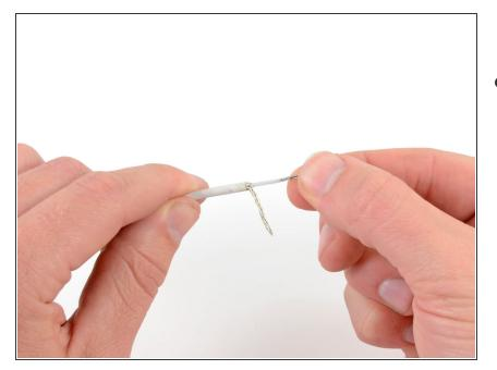
As before, twist the center wire strands tightly into a single twisted strand.
