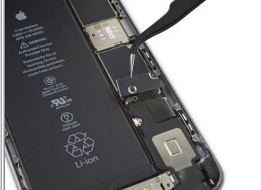
• Remove the battery connector bracket.
