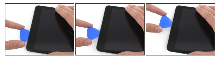
Pull the pick out slightly, and slide the very tip gently along the top of the front-facing camera section of the top edge.
