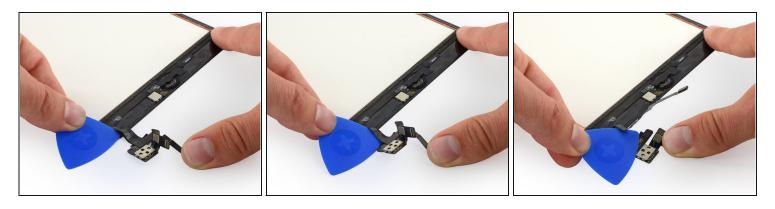
Use an opening pick to break up the adhesive holding the home button ribbon cable to the digitizer cable.
