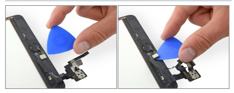
Use an opening pick to lift the home button control hardware off the back of the front panel.
