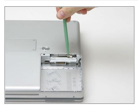
Use a spudger or flathead screwdriver to disconnect the Airport antenna from the card.
