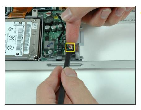
Use a spudger or the tip of your finger to disconnect the hall effect sensor cable from the DC-to-DC board.
