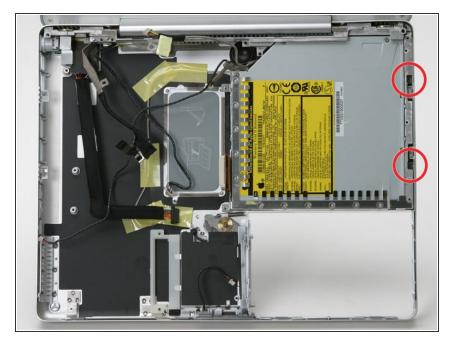
Remove the two recessed Phillips screws on the right side of the optical drive.
