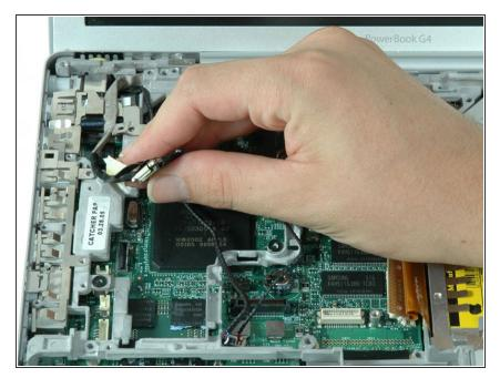
Peel up the yellow tape securing the display data cable to the metal framework, and deroute the display data cable from its slot in the framework.
