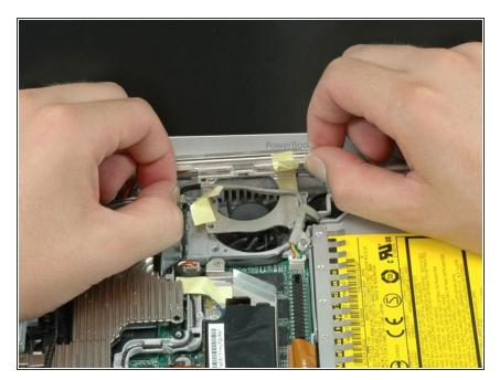
Lift up the inverter cable with one hand, and carefully thread it around the heat sink. The inverter cable is still attached to the logic board, so be careful not to put too much strain on the cable.
