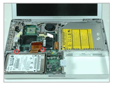
Remove the two Phillips screws securing the hard drive bracket to the metal framework.
