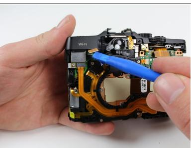
Disconnect the cable on the back of the camera to the left of the viewfinder by lifting it up vertically using a plastic opening tool.
