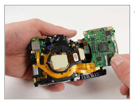
Lift the motherboard out of the camera.
