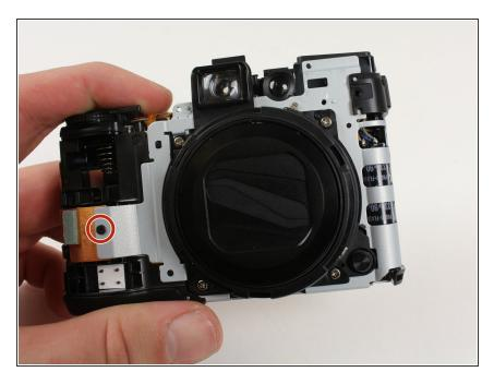
Remove the black 3.8 mm screw on the far left side using a Phillips #000 screwdriver.
