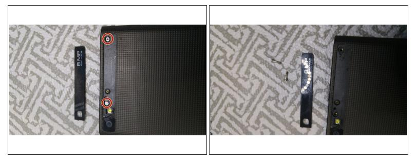
• The screws are behind the sticker beside the camera. Heat the sticker and use a knife to pry under the sticker to remove it. There are 2 screws which you need a T6 torx screwdriver to remove.
