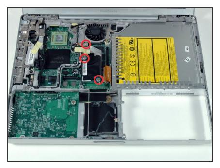
Remove the three Phillips screws securing the modem and modem shield to the logic board.
