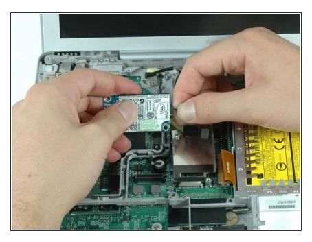
Turn the modem over and disconnect the RJ-11 cable.
