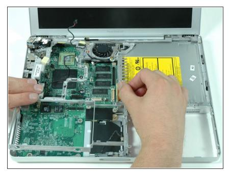
Pull back on the orange optical drive cable with one hand, and use your other hand to lift the front section of the metal framework over the optical drive cable.
