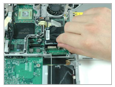
Disconnect the modem from the logic board by lifting the bottom edge of the modem. Don't remove the modem entirely just yet as it is still connected to the RJ-11 board.
