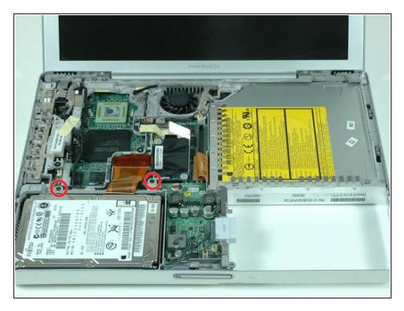
Remove the two Phillips screws securing the hard drive bracket to the metal framework.
