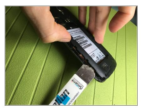
With the help of a thin instrument, unhook the central structure anchored to the external profile
