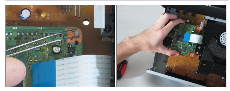
• Using <u>tweezers</u> or pliers, squeeze the tabs of the plastic fasteners together. While doing this, gently lift up on the motherboard until the fasteners are released.
