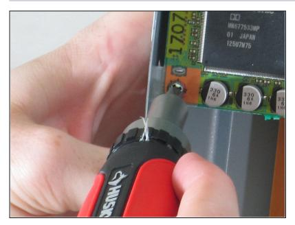
• Remove the two screws securing the motherboard using a philips screw driver.
