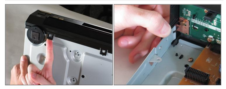
• Lift up the five tabs securing the front panel to the chassis. There are three on the bottom, and two on the inside edges of the panel. Panel should then lift off the player.
