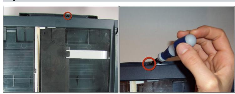
• Once the scanner lid is removed, use the Philips #1(Torx on some printers) Screwdriver to remove the screw.
