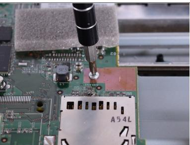
Use the PH1 screw driver to remove the three screws on the motherboard.
