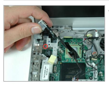
Lift the RJ-11 board up from the left side, and remove the single Phillips screw hidden beneath.
