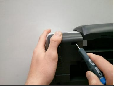
Insert the pointed end of a spudger into the hole on the bottom right corner of the printer and pry out the tab.
