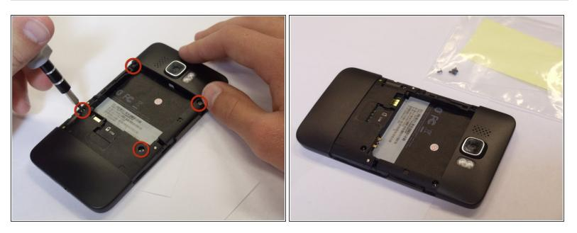
Remove the four black 3.5mm T5 screws from the back of the phone.
