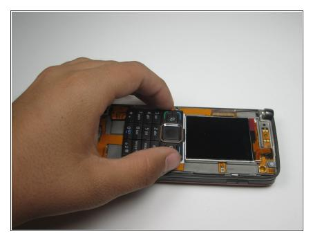
With the front cover off, the screen and keypad should be loose.
