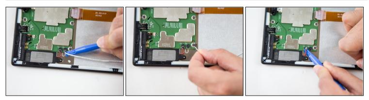
• Disconnect the connectors using the plastic opening tool.
