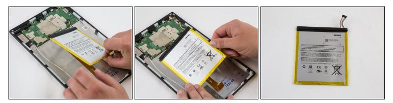
• Inspect battery for any leakage.
