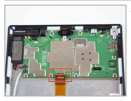
• Lift the ZIF connector up to disconnect from the motherboard.
