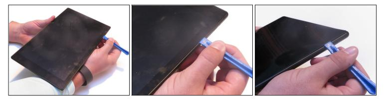
$\Delta$  Avoid prying near bottom right hand side due to LCD Connector
