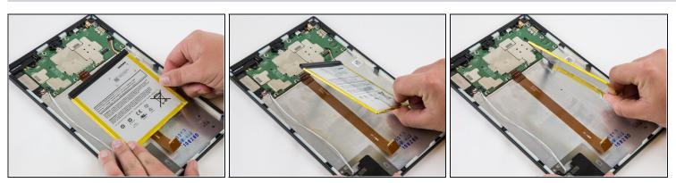
A Make sure all the adhesive is removed before trying to lift the battery from the case.
