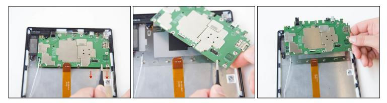
• Lift and pull the motherboard down, gently, towards the case using the tweezers.
